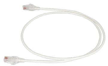
RDC 6 Modular Patch Cord, white, 25', reduced diameter, 28 AWG, cat6 channel four-pair UTP stranded PVC/CM.
