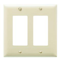
The TradeMaster® thermoplastic 2-gang decorator wall plate provides maximum durability in plastic wall plates. Selfextinguishing nylon construction makes thesewall plates virtually unbreakable. They are 3/16 of an inch higher and wider than typical plastic wall plates - not enough to be apparent to the eye, but the extra size cuts cost by reducing dry wall rework.
