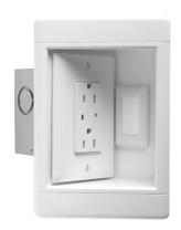
Allows for snug-to-wall placement of your flat-screen TV and handles up to 12 multimedia connections. TV Frame supports line and/or low-voltage devices. Accepts all Pass and Seymour keystone low-voltage connectors, including Cat 5e and F-Connectors, as well as RCA and audio binding posts (not included).
