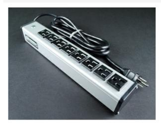
Eight outlets, rugged gray aluminum housing, 15A. 6' (1.8m) 14/3 SJT black cord with NEMA5-15 plug. Length 13" (330mm). Receptacle center-to-center 1 1/4" (32mm). Snap-on, slide-off mounting.
