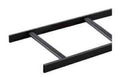
Universal Style Tubular Runway features 1 in x.5 in tubular cross slats that are welded between .375 x 1.5 in high tensile tubular steel stringers. Cross slats feature rounded edges for cable protection. Standard length is 9ft 11 in, and widths from 6 in to 24 in. Available in rust-resistant, powder coated black finish only. UL listed.
