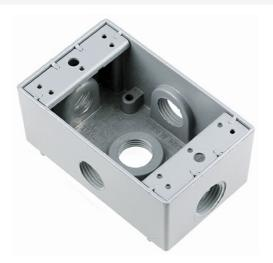
Weatherproof 1 Gang Box, 5 Hole 3/4"", 16.8 Cu. In., Gray (1 Hole Each End, 1 Hole Each Side, 1 Hole in Back)
