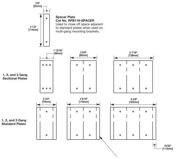
Standard Plates extend 15/32" [11.9mm] on each side wider than sectional plates. Step 11 Determine device plate required to close off wiring compartments. Sectional (1-13/16" [46mm] wide) or standard device plates may be used with multi-gang mounting plates.
