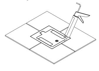
Step 20 After concrete or terrazzo has cured, mount cover to box as shown in Steps 14 and 15. Apply sealing compound around perimeter of cover, as shown in Step 18.
