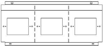
Step 12 Mount blanking plates and spacers between standard size plates to close off any gaps or openings. Typical layouts are illustrated below.
