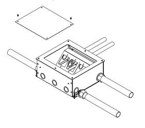
Step 2 Level & anchor box. Top of box must be flush with concrete pour. Use screws, nails, or wire to prevent box from floating during pour.
