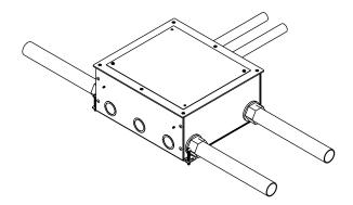
NOTE: For use in bare concrete or terrazzo floors, replace mudcap with part number: RFB119-PAN. (Sold separately.) (See Step 19.) Step 5 Screed to top of box surface. Hand troweling recommended near box edges.
