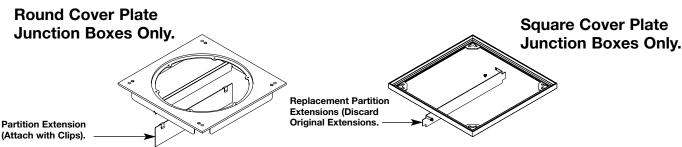
Reassemble Junction Box Components and Install New Tape Around Cover Plate.
