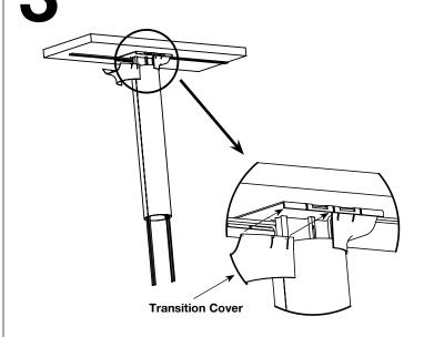
Snap boot halves together around channel.
