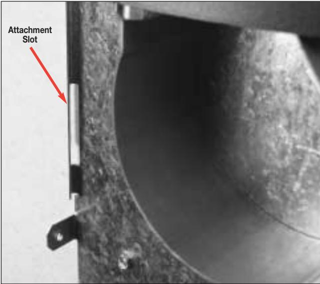
**Step 6.** To attach DS4011 Cover: Hook the inside corner then rotate down and snap into place. The DS4017 and DS4018 Covers snap straight on. Covers overlap raceway cover by approximately 3/8" [10mm].
