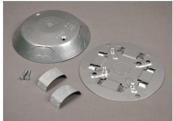
May be used with 1500 and/or 2600 Series Raceway as a cross, tee, or elbow. Cover has 1/2" trade size KO. Base has 1/2" and 3/4" concentric KO to enable connection to floor, outlet boxes or under floor duct systems (use Chase nipple not included). Two 2600WC Wire Clips included.
