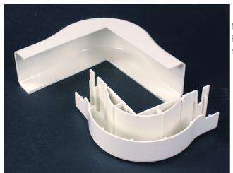
Makes right angle turns around internal corners of 2900 Series Raceway running at right angles. Maintains 1 1/4" (32mm) bend radius when installing UTP and fiber optic cable.
