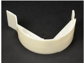
Radiused insert for the 4011 Flat Elbow and the 4015 Undivided Tee. Provides 2" (51mm) cable bend radius control for UTP, STP or fiber optic cable installations. Ideal for new and retrofit applications whether the cable installation is lay-in or pull-through.
