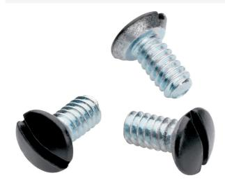
Oval head milled slot 1/2-inch long, 6x32 thread. Standard size for duplex receptacles and toggle switch wall plates. .
