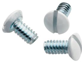
Oval head milled slot 1/2" long, 6x32 thread. Standard size for duplex receptacles and toggle switch wall plates. White.
