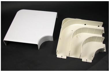
90 degree flat corner, with integral dividers, that provides a 2" (51mm) cable bend radius for UTP and fiber optic installations. Ideal for lay-in or pull-through installations.
