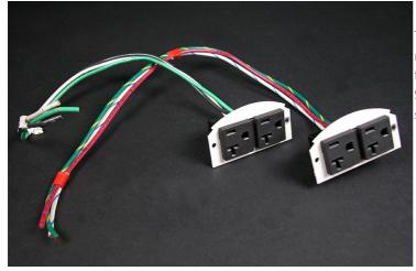
Two (2) proprietary 20A duplex power receptacles with mounting plates and 25' leads. Designed to fit in either of the two side compartments in both the 6ATC and the 8ATC Series Poke-Thru Devices. Receptacle can be wired as a standard or isolated ground device.
