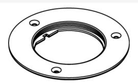
Brass communications or power cover plate with 2 5/8" (67mm) threaded opening for tile. Sold without abandon plug. NOTE: For carpet or tile installations. All cover plates are furnished with gasket and three screws. The 895P Polycarbonate Series Cover Plates must be field modified for dual service.
