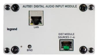
The Digital Audio Input Module provides the Digital Audio System with access to streaming digital music and services. Content is accessible from any zone within the system, or from all zones simultaneously. The AU7001 includes built-in access to I
