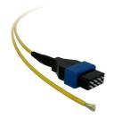
acclAIM Laser Cleaved, 8 Fiber, Splice-On Pigtail is used to splice with existing fiber trunks or new multifiber cable, enabling quick and easy cable runs and connection to the patch panels. The connectorized acclAIM end has been pre terminated in the factory for maximum reliability and quality results. The Laser cleaving simplifies fiber splicing which greatly decreases labor and cost.
