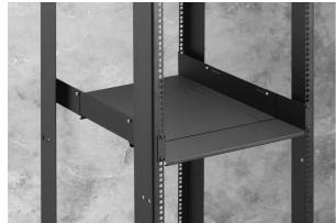
Equipment shelves mount to 19" or 23" equipment racks. Heavy -duty 16-gauge steel accommodates heavy equipment. Patented shelves can be mounted upside down. Shelves are vented to allow air flow beneath mounted equipment. Black.
