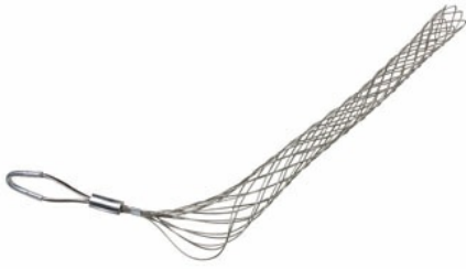
FC3500F: Standard Duty, Closed Mesh, Offset Eye Grips, Cable Diameter 3.50 - 3.99 inches, Bale Length 9-in, Mesh Length 28-in, Break Strength 5040 lbs.
