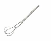
FCSD30LB: Service Drop, Closed Mesh, Locking Bale, Cable Diameter 0.30 - 0.43 inches, Bale Length 11-in, Mesh Length 5-in, Break Strength 500 lbs.
