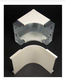
Full capacity, divided internal elbow. Provides 2" (51mm) cable bend radius control for UTP, STP and fiber optic installations. Ideal for new installations whether the cable is lay-in or pull-through.
