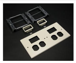
Accepts 15A and 20A duplex receptacles and 106 style frame. Includes mini adapter that accepts Pass and Seymour Activate inserts or Wiremold Open System communications modules. NOTE: Certified to Canadian Safety Standards for sale in Canada. When ordering these products, change the "V" color prefix to "CV" or the "G" color prefix to "CG" to denote the Canadian versions.
