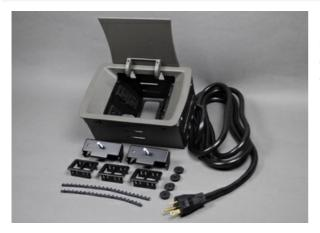
Cord-ended with gray, flush cover. Unit comes with two 20A gasketed prewired receptacles with a 12' (3.65m) 14/3 SJT black cord. Includes adapter for Ortronics Series II and TracJack inserts. Communication modules sold separately.
