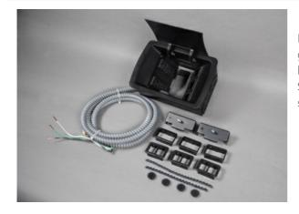
Field-wired with black, flush cover. Unit comes with two 20A gasketed prewired receptacles with a 3/8" (9.5mm) diameter 6' (1.83m) flexible whip. Includes adapter for Wiremold CM Series Open System communications outlets. Communication modules sold separately.
