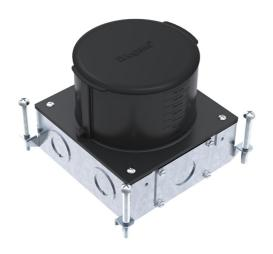
Rectangular dual service metal concrete floor box with a nonmetallic top that allows for concrete pours between 4" thick to 6" thick. Graduated markings on the inside and outside of the box indicating volume capacity, as well as the depth of concrete pour. Box accepts 2HUB to allow 2" conduit feeds (sold separately) while maintaining a 4" deep concrete pour. Box includes: (1) Reusable concrete cap (2) Removable knockout plates to allow the 2HUB to be attached.
