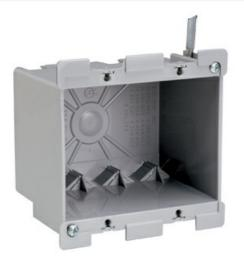
Double Gang, Old Work Switch and Outlet box with swing-bracket for mounting, adjusts from 1 1/4 to 1/8. It has four Auto/Clamps for each end. It has a durable, impact-resistant thermoplastic box. The metal swing bracket is for quick mounting in existing walls.
