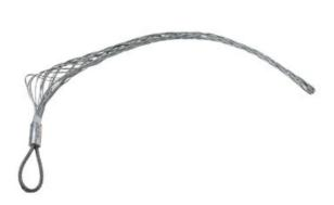
Double Weave, Long Length, Closed Mesh, Offset Eye. Cable Diameter - 1.500-1.740-inch, Mesh Length - 26-inch, Break Strength - 7,400 lbs.
