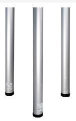
Satin anodized finish. Nominal wall thickness .060" (1.5mm). Length: 10' 3" (3.1m). Provided with one 1/2" (12.7mm) trade size KO at base. T-bar mounting hardware, ceiling trim kit, foot assembly, and grommet included. Feed box not furnished.
