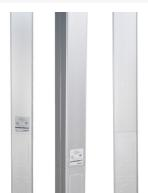
Two-compartment pole. Nominal material thickness .050" [1.8mm]. Length: 15' 5" [4.7m]. Furnished unwired without outlets. Two 8" [203mm] removable covers with KOs for modular jacks and modular furniture communication outlets. Mounting hardware, entrance end plate and ceiling trim plates furnished. NOTE: Custom options - features such as colors or other lengths [20' [6.1m] maximum] available on custom orders.
