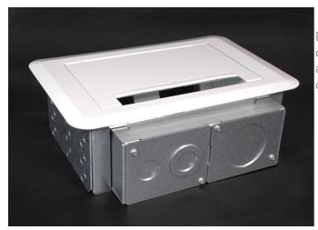
Designed to fit and be concealed behind 42" or larger flat screen displays. Can be installed in both new work and old work applications. Has 4 NEMA size openings for power, communication, or A/V devices.
