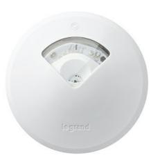
The LMDL-600 is a wireless open loop photo sensor that measures the daylight contribution in order to automatically switch or dim multiple zones of lighting. It is part of the wireless Digital Lighting Management (DLM) system and sends light level signals to control loads connected to DLM on/off or dimming room controllers.
