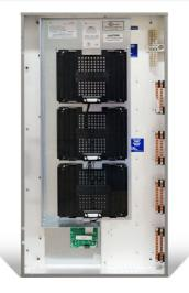
The InFusion LiteTouch Retrofit Insert is designed to easily fit into a LiteTouch®/Savant® enclosure and can house up to three separate control modules or up to 36 loads per enclosure. This insert features module locking mechanisms for improved in-field plug-and-play installation and service, allowing modules to be quickly replaced without affecting load connections to the system.
