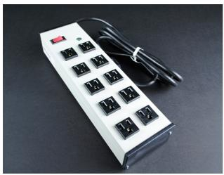
Ten outlets, rugged gray aluminum housing, 15A, lighted switch. 6' (1.8m) 14/3 SJT black cord with NEMA5-15 plug. Length 13'' (330mm), width 3 1/2'' (89mm). Receptacle center-to-center 1 15/16'' (49mm). Snap-on, slide-off mounting.
