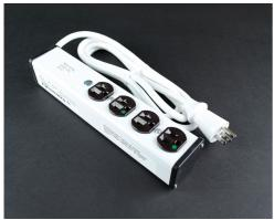
Four outlets. Rugged white aluminum housing. 6' (1.8m) 14/3 SJT white cord with NEMA5-15 plug. Length 10 3/4'' (237mm). Receptacle center-to-center 1 1/2'' (38mm). Snap-on, slide-off mounting. cTUVus Listed as Medical Electrical Equipment. NOTE: Suitable for use where Article 517 of NEC requires Hospital Grade Outlets.
