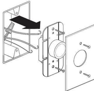
When replacing existing devices, label wires before disconnecting. Disconnect old device.
