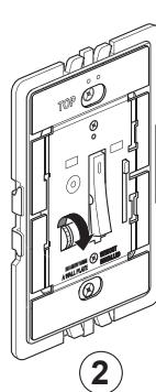
Replace cover assembly. Hook at the top and rotate down to snap into place. Note: Sliders need to be in the same position during cover re-assembly.
