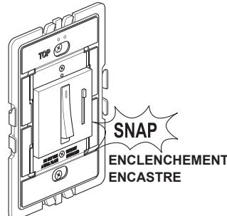
**NOTE** - If you need to remove dimmer after snapping into frame, first remove frame from wall box to access the four locking tabs on the back of the dimmer. Insert a flat screwdriver to depress tabs as you apply pressure to push dimmer out.
