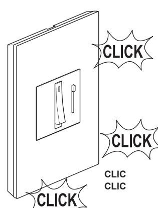
**NOTE -** To remove wall plate, insert a small, flat screwdriver in notches
