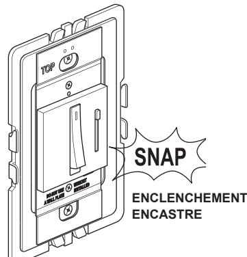
**NOTE -** If you need to remove dimmer after snapping into frame, first remove frame from wall box to access the four locking tabs on the back of the dimmer. Insert a flat screwdriver to depress tabs as you apply pressure to push dimmer out.
