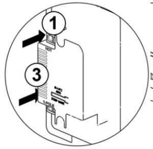
**NOTE** – To remove wall plate, insert a small, flat screwdriver in notches on wall plate and twist gently to pry from frame.
