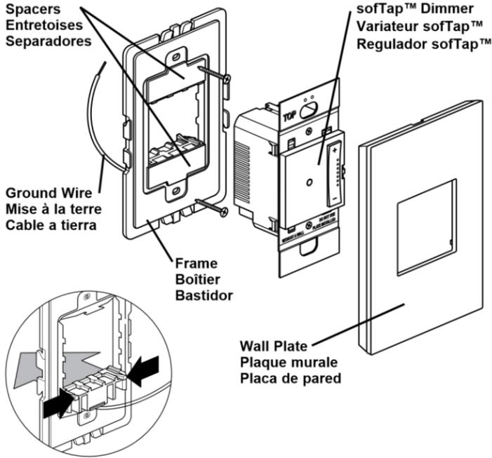
**Remove spacers from the frame.** Since this dimmer fills the frame completely, you will not need the spacers. From the back of the frame, pinch the tabs on the spacer to release.
