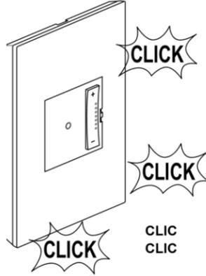
**NOTE** – If you need to remove dimmer after snapping into frame, first remove frame from wall box to access the four locking tabs on the back of the dimmer. Insert a flat screwdriver to depress tabs as you apply pressure to push dimmer out.
