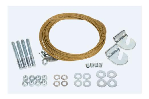
SZMCKIT is a 10' long, gold 4-way seismic kit. Kit includes 4 lengths of cable. 3/8" stake eyes, bent on a 45 degree angle, are factory-installed on one end. The kit includes 2 URCR clips, 4 oval sleeves and 4 wedge anchors.
