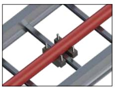
STEP 3 Position cap and finger tighten all four nuts. Then 1/2 turn with wrench.
