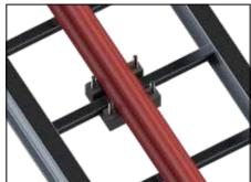
STEP 3 Position cap and finger tighten all four nuts. Then 1/2 turn with wrench.
