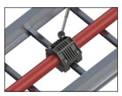
Cable Cleat — Trefoil STEP 1 Install rung spacer if required
