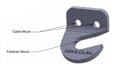
The URCR clip is designed for use in attaching seismic cable bracing to equipment and trapeze supports. This clip can be used in both new and retrofit installations. The fitting is slotted to allow an existing fastener to be loosened and the URCR clip positioned without removal of the fastener. The two cable mounts will accept Gold, Orange and Green cable. The UL listing applies to Gold and Orange cable assemblies only.
