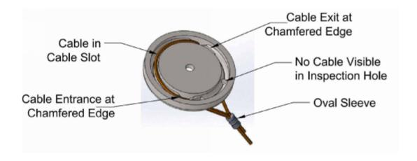
The NPC clip is specifically designed to reduce the prying effect on fasteners. The cable is nested in the groove provided and exits through two chamfered slots to prevent damage to the outer fibers of the cable. An inspection hole is provided to ensure that the cable is placed in the correct position within the groove.
