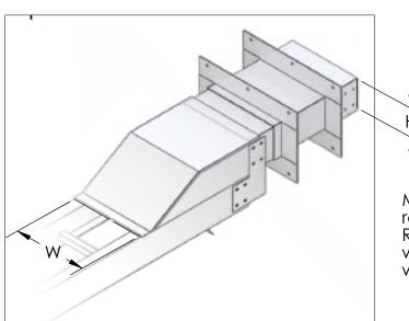
Makes ladder tray wall penetrations weather resistant to minimize water intrusions. Removable cover/shield fastens to tray and wall penetration sleeve for the utmost in weather protection.
