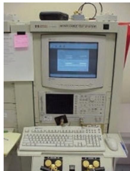
Comparisons were made for NEXT, FEXT, return loss and input impedance.
