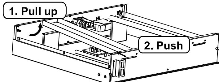
**NOTE:** To install the second branch of batteries, repeat the same procedure on the battery fixing plate on the right side of battery box
