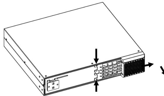
Step 4: Remove the metal top cover of the battery box by unscrewing the 6 screws present on the two sides (3 on the right side + 3 on the left side) and the 3 screws on the top and the 4 screws on the back side.
