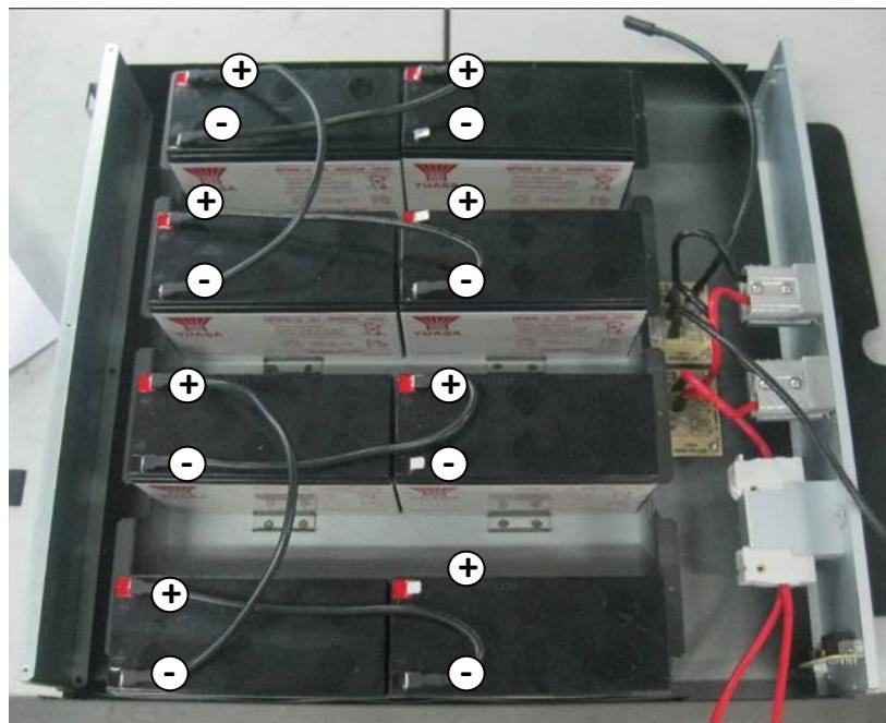
**NOTE:** The cable connection from the external battery connector to the PCB is already present inside the battery box. All the other cable connections should be made as shown on the wiring diagram.
