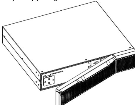
Step 3: Remove the fixed part of the front panel by removing the 2 screws present.
