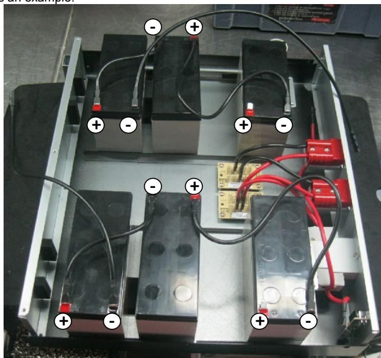
**NOTE:** The cable connection from the external battery connector to the PCB is already present inside the battery box. All the other cable connections should be made as shown on the wiring diagram.
