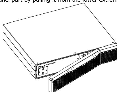
Step 3: Remove the fixed part of the front panel by removing 2 screw present.
