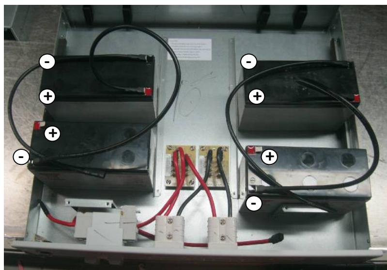
**NOTE:** The cable connection from the external battery connector to the PCB is already present inside the battery box. All the other cable connections should be made as shown on the wiring diagram.
