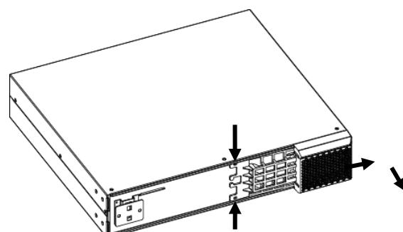
Step 4: Remove the metal top cover of the battery box by unscrewing 8 screws present on the two sides (4 on the right side and 4 on the left side), 3 screws on the top and 4 screws on the back side.
