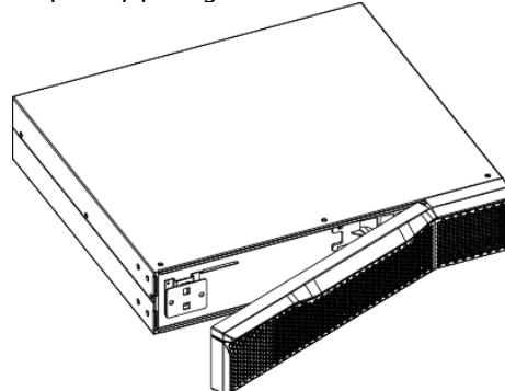
Step 3: Remove the fixed part of the front panel by removing the 2 screw present.
