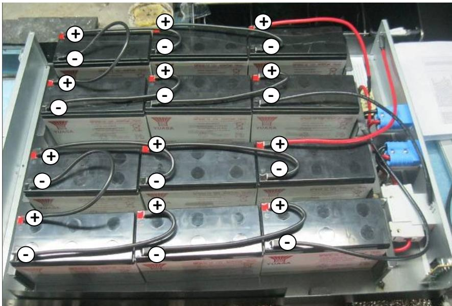
**NOTE:** The cable connection from the external battery connector to the PCB is already present inside the battery box. All the other cable connections should be made as shown on the wiring diagram.
