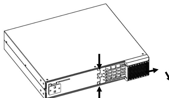
Step 4: Remove the metal top cover of the battery box by unscrewing 6 screws present on the two sides (3 on the right side and 3 on the left side), 3 screws on the top and 4 screws on the back side.
