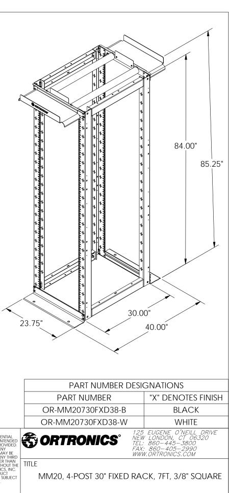
TESTED TO UL2416 WITH A WEIGHT LOAD OF 2000LBS.
