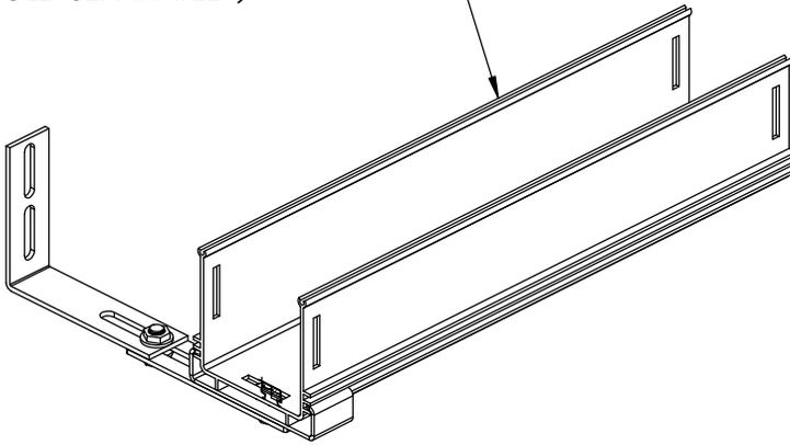
TYPICAL RACEWAY MOUNTING EXTENSION BRACKET CONFIG.
